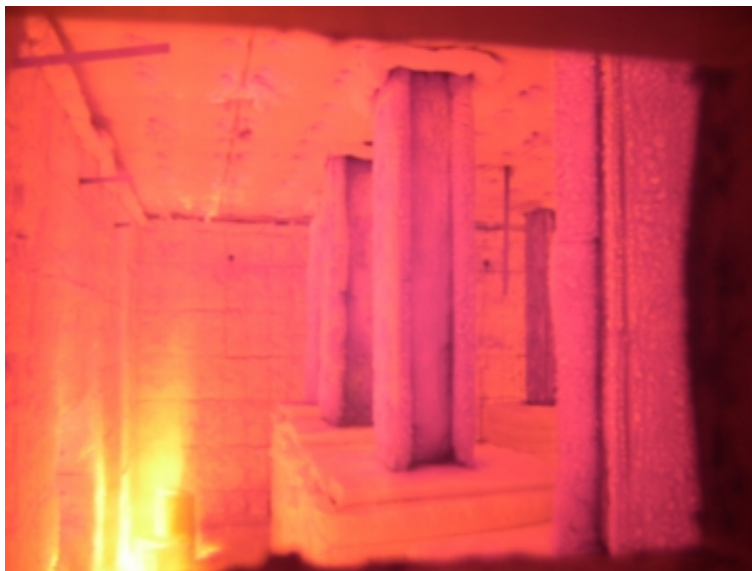
Char Forming (W8×31 in Center of Picture)
