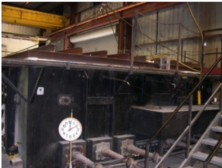
Furnace Extinguished After 2 Hour Exposure
